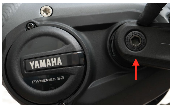
Loosen the hexagon head screw (8 mm) of the crank and pull off the crank with a crank puller.
