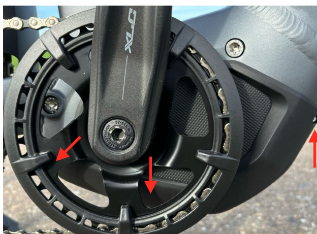
Loosen the 3 hexagon head screws (3 mm)
