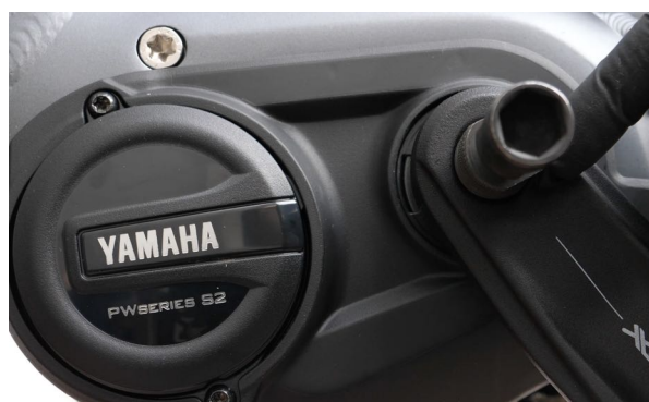
Loosen the hexagon head screw (8 mm) of the crank and pull off the crank with a crank puller.
